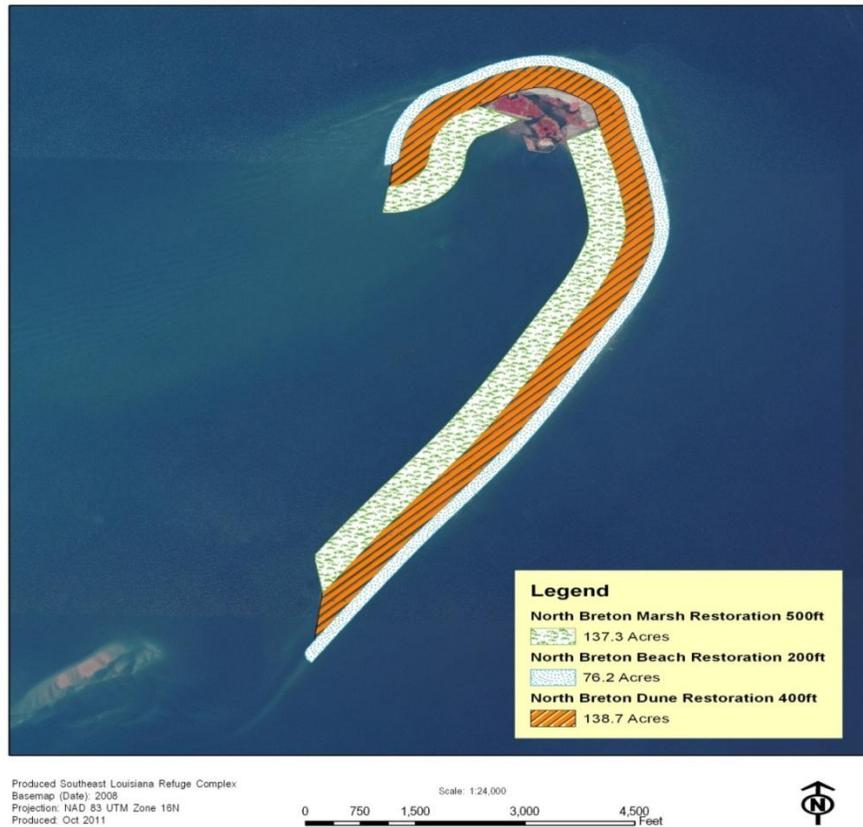
**Figure 9-7. Conceptual design for North Breton Island Restoration.**
