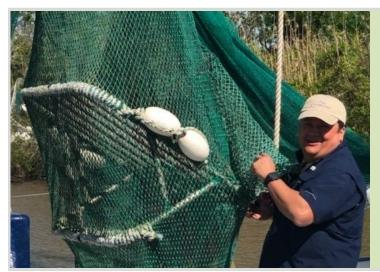
NOAA Fisheries Service Gear Monitoring Team staff member, Peter Nguyen, displays a fixed angle TED design. This design is likely to be tested with a 45° angle in conjunction with other modifications, such as reduced bar spacing of 2.5". Photo credit: NOAA
