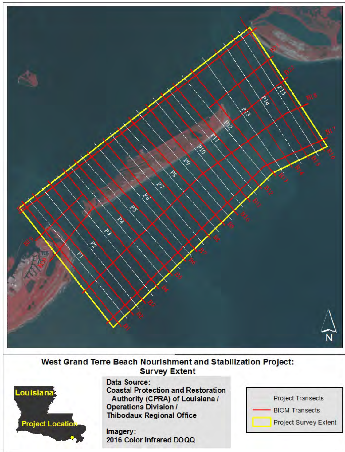
Figure 2. Survey extent and transect lines for bathymetric and topographic survey.
