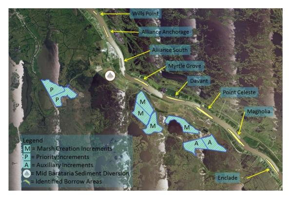
Figure 22. Individual marsh creation increments that are part of the Large-Scale Marsh Creation – Component E project. The increments being brought forward for Phase II planning are labeled as priority increments (P).
