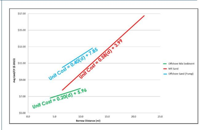
Figure 4. Cost versus Distance Pumped by Sediment Source (CPRA, 2017 Appendix A)
