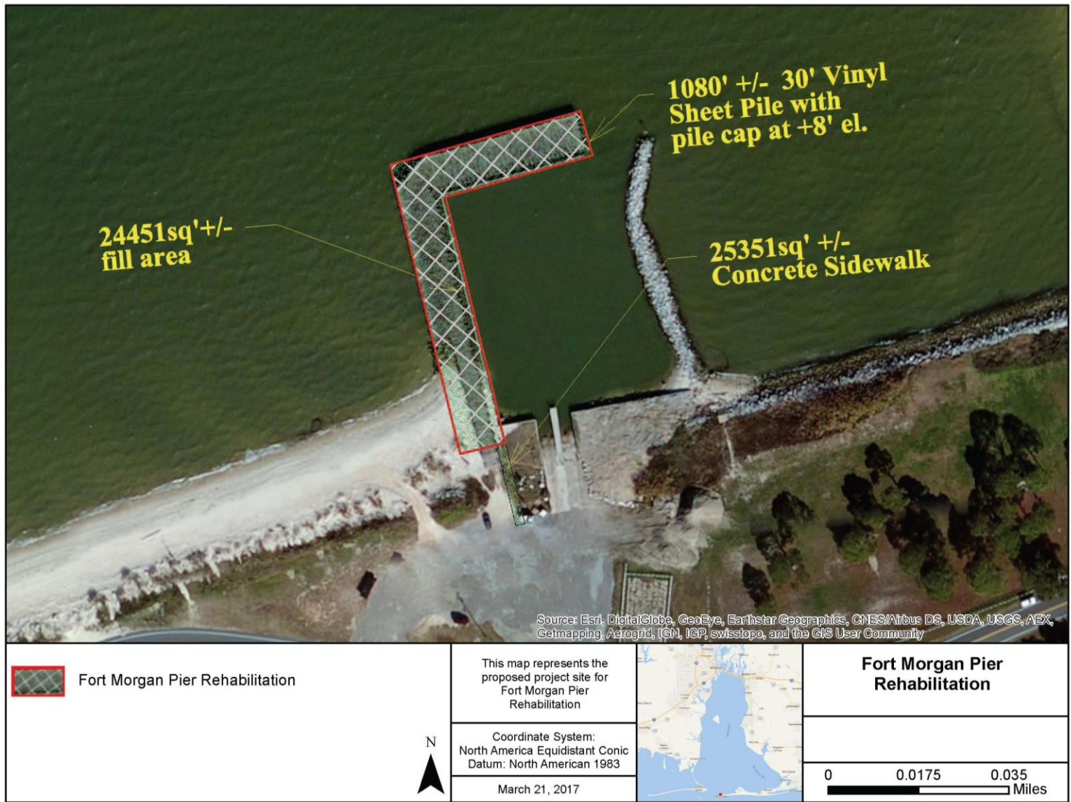
Figure 2-3: Fort Morgan Pier Rehabilitation
