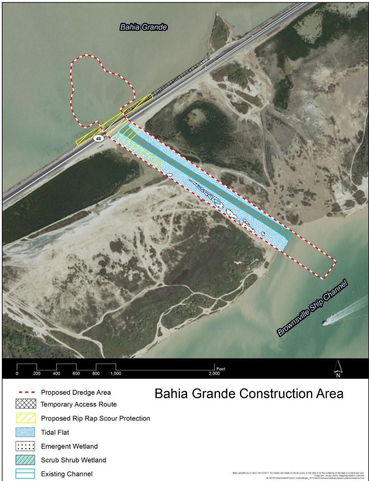
Figure 5-4. Map showing the location of the existing pilot channel and proposed expansion of the channel.
