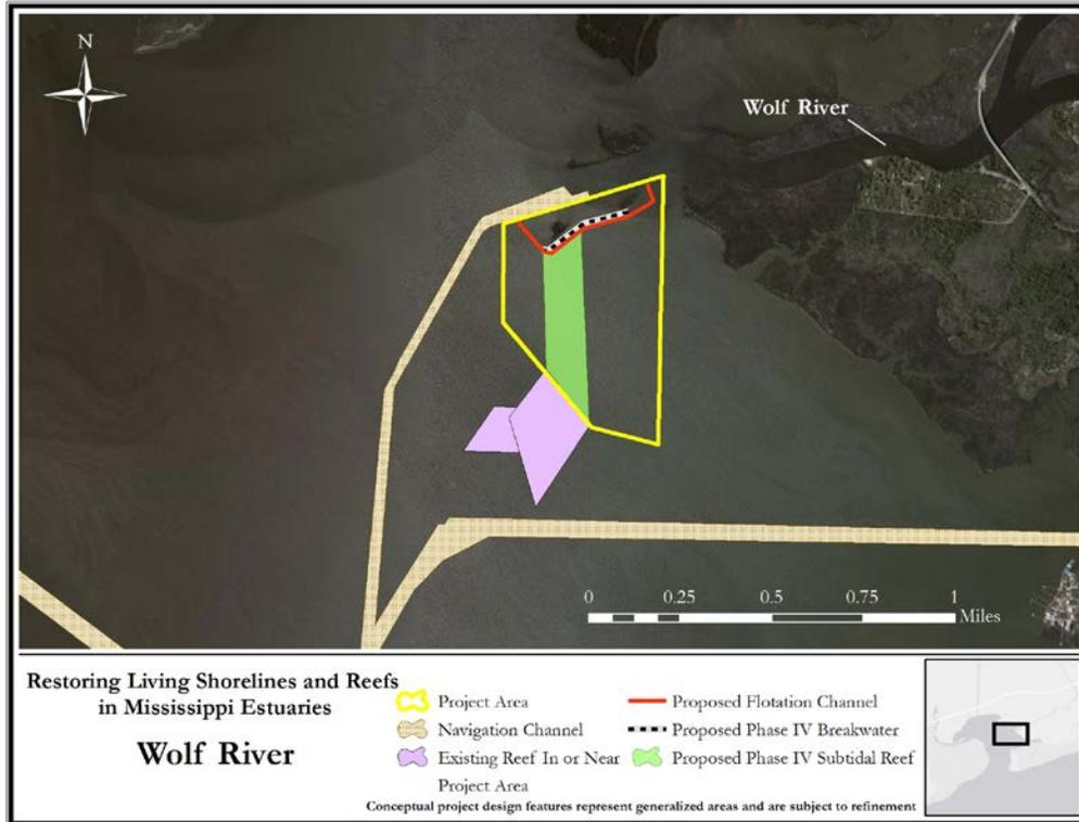
St. Louis Bay Living Shoreline (Figure 6-9): Would include the construction of approximately 10,812 ft. of breakwater in St. Louis Bay. Conceptual site locations for the breakwater and temporary flotation channels are depicted in Figure 6-9 and are subject to refinement. Temporary flotation channel conceptual locations and footprints have been included for the purpose of estimating the maximum impact, but may be avoided depending on project design and/or construction timing.
