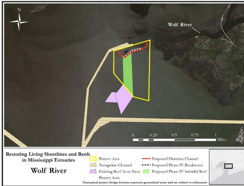
St. Louis Bay Living Shoreline (Figure B- 10): Would include the construction of approximately 10,812 ft. of breakwater in St. Louis Bay. Conceptual site locations for the breakwater and temporary flotation channels are depicted in Figure B- 10 and are subject to refinement. Temporary flotation channel conceptual locations and footprints have been included for the purpose of estimating the maximum impact, but may be avoided depending on project design and/or construction timing.
