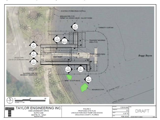
Figure 4-11 Conceptual drawings for the boat ramp and dock at Lincoln Park
