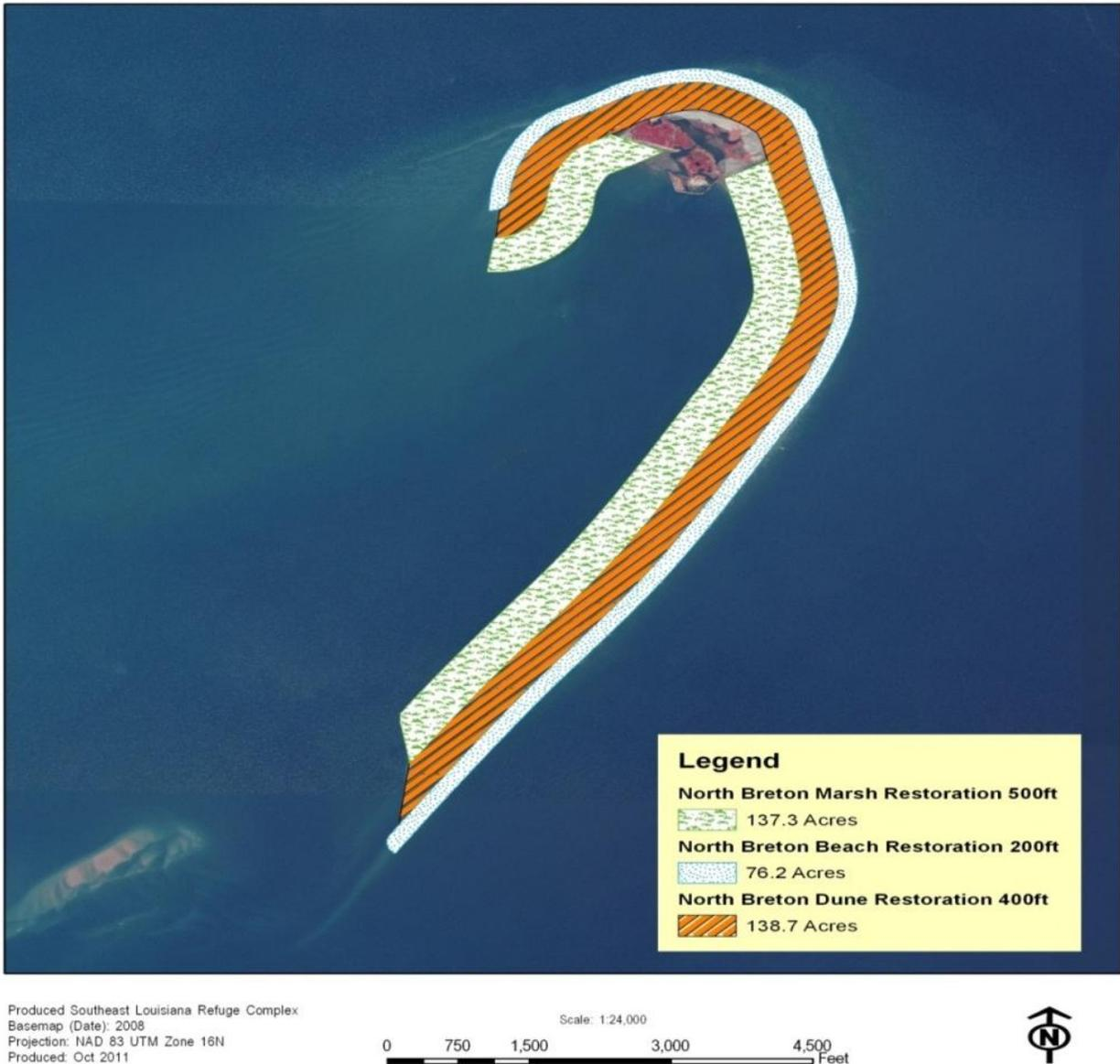
**Figure 9-8. Conceptual design for North Breton Island Restoration.**
