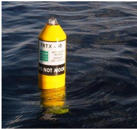
**Figure 8-4. Example of a USCG approved marker buoy.**
