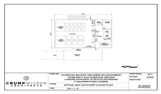
Figure 9-22. Floor plan for the Plaquemines Parish facility.
