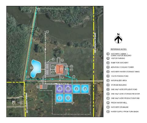
Figure 9-19. Proposed site plan for the Calcasieu Parish facility.
