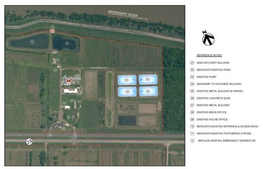
Figure 9-21. Site plan for the Plaquemines Parish facility.
