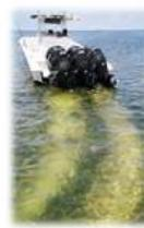
Blowhole created by a propeller
