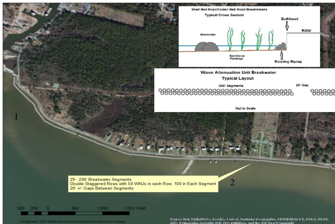
**Figure 11-3. Proposed Project Layout – Shell Belt and Coden Belt Roads Living Shoreline**
