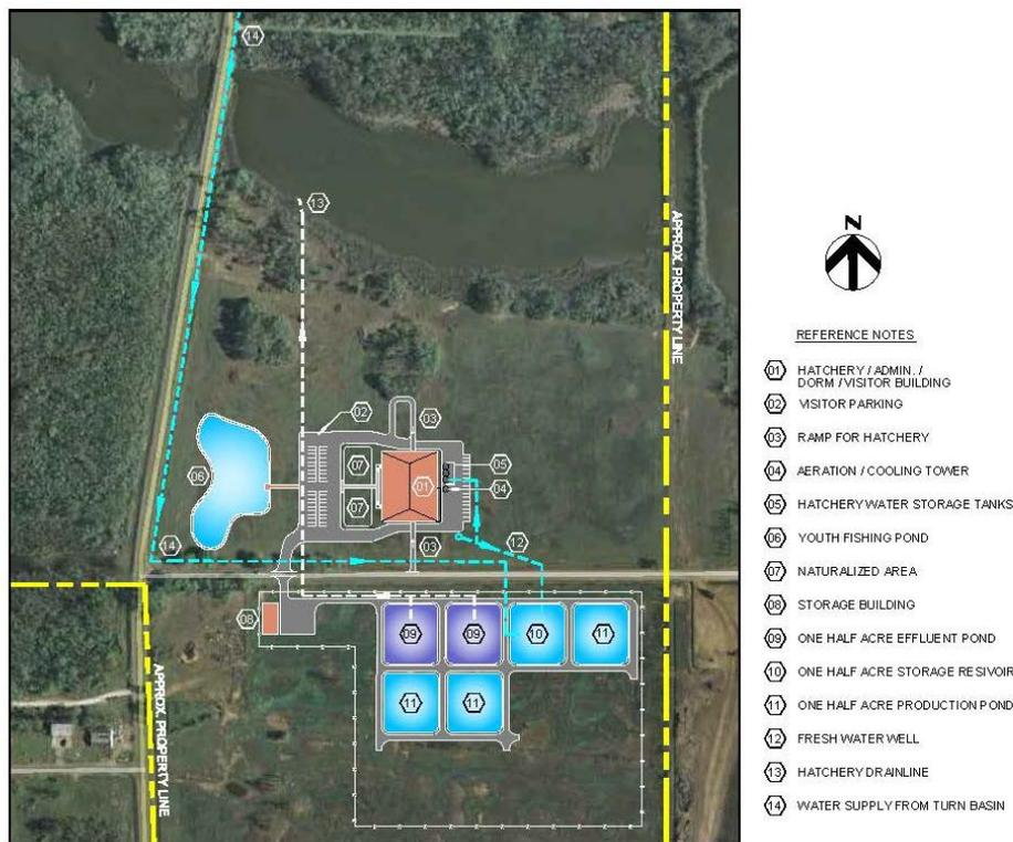
**Figure 9-20. Proposed site plan for the Calcasieu Parish facility.**
